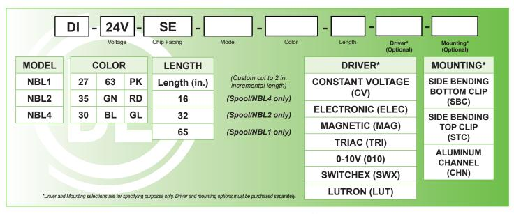
Example: DI-24V-SE-NBL2-35-16-CV-TBC = Diode LED, 24V NEON BLAZE<sup>m</sup> 2.44 w/ft. 3500 CCT, 16.4' long, 96" Lead Wire, and with a Constant Voltage Driver, and Top Bending Bottom Clips.
