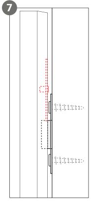
Fasten the channel to the mounting clip on the vertical surface with the vertical bracket resting above the mounting clip.
