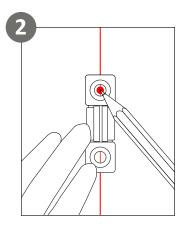
Mark holes where the mounting clip will be fastened. Fasten two clips per channel, each 1/4 distance the full length of the channel from each end. E.g. if the channel is 40 in. long, mount each clip 10 in. from each end.
