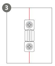
Fasten the mounting clips with an electric drill and mounting screws. Use applicable screw anchors if required for installation.
