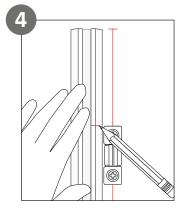
Hold the channel up to the guide and mounting clip. Mark the channel where the top edge of the mounting clip will be located.
