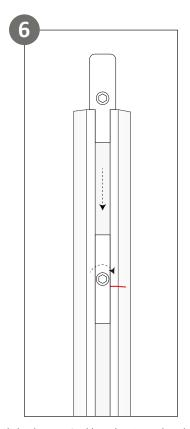
Slide the vertical bracket into the channel and tighten with the allen wrench. Ensure the bottom edge of the allen hardware meets the mark previously noted on the channel.
